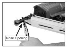
Figure 7. Nose opening for clearing a jammed nail.
